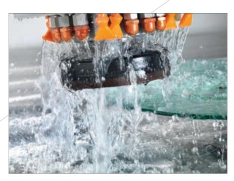
To ensure that the highest quality standards are achieved in bevel machining operations, Diamut has implemented numerous tests on products involved in this process, to ensure that the company continues to offer the best sequence of grinding wheels available. Over time, Diamut has developed wide range of gouge angles available on their grinding wheels, so that both internal and shaped bevels can be carried out on monolithic, layered and laminated glass.
