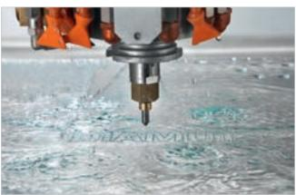
The extensive Diamut range also includes writing bits with a 2 mm to 10 mm diameter with 1/2" GAS support.
