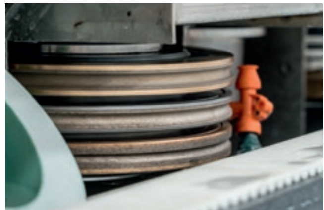
Maximum flexibility thanks to the possibility of creating a version with up to 4 over-stuck grinding wheels, to allow a quick thickness change of the glass to process.
