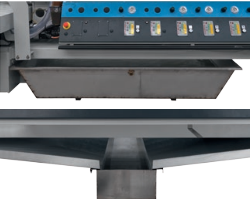
The drainage of waste waters is carried out in a simple and effective way.
