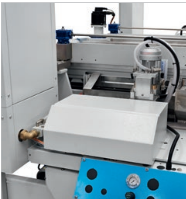
Working up to 10 m/min Electronic corner cutting spindles to execute chamfers and corners up to 10m/min.
