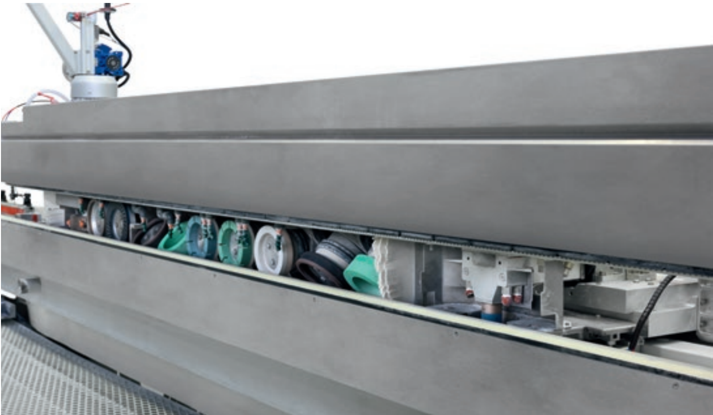
The corner-rounding system is fully integrated in the crosspiece structure.
