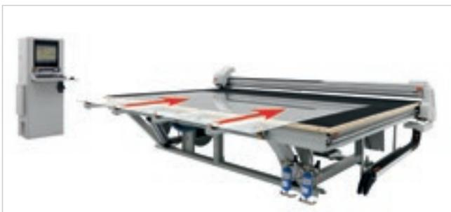
The drop-down feet automatically move back to their safety position for the cut cycle start. The operating head automatically begins the cutting cycle.
