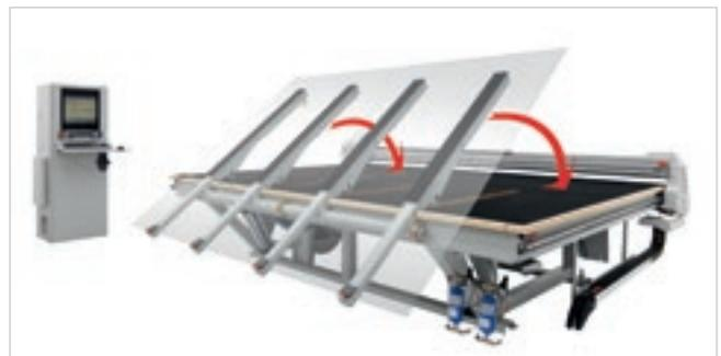
The tilting arms automatically put the glass sheet in the working position.
