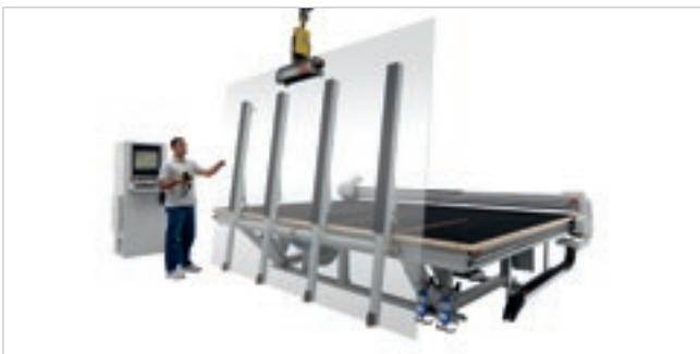
The tilting arms automatically put the glass sheet on the work table.
