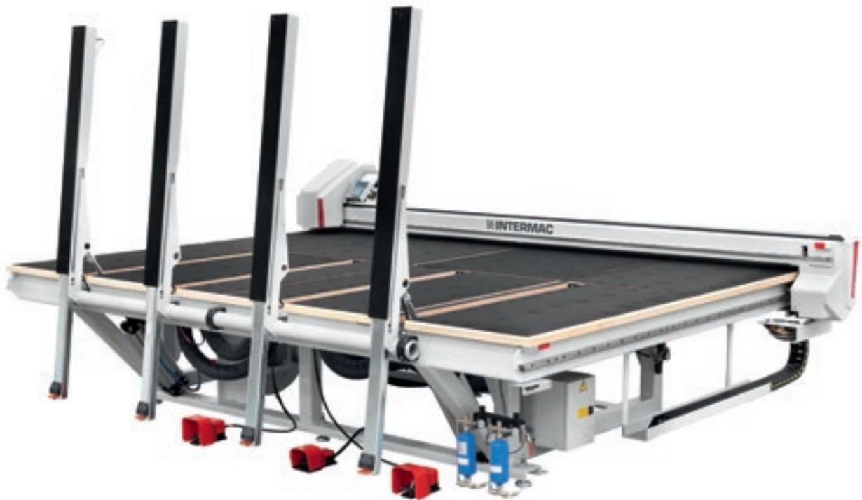
The Genius RS-A is compact in terms of both width and height, thanks to the tilting arms that only extend to a maximum of 2.5 metres.
