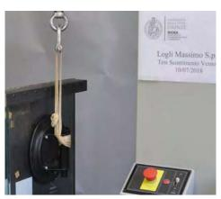
Thanks to the extensive testing, the recommended safe working values for normal operating conditions have been calculated: for each device, under different conditions of use, the recommended value represents the minimum measured value, reduced by a safety coefficient of 1.5.
