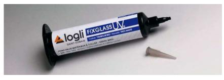
Technical data: Colour: transparent Resin: Urethane acrylate Viscosity: thixotropic (very dense) Consistency: elastic Flash point [°C]: > 93 Density [g/cm<sup>3</sup>]: about 1.1 UV (UV-A 60 mW/cm<sup>2</sup>): 5 sec. Max. catalysing thickness [mm]: 5 Visible light (400-480 nm) [s]: 10 Fillable thickness [mm]: 0.09-0.5 Final performance [h]: After 12 hours Temperature resistance [°Cl: -50-150 Hardness [Shore A]: 60-70 Retraction [Vol-%]: 4.3 Water absorption [mass-%]: < 0.8
